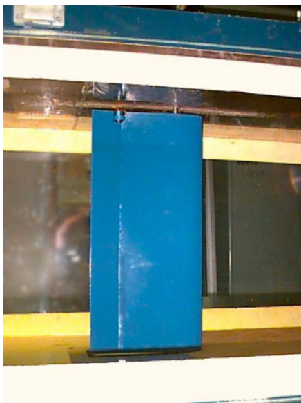
(a) Full span typical section model
